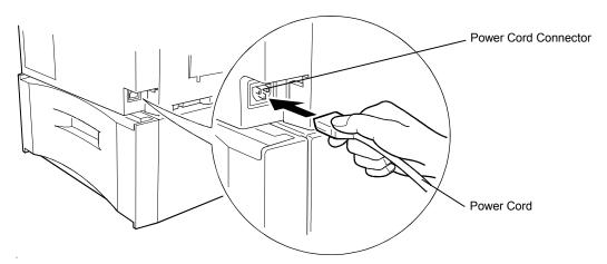
2. Connect the other end of the power cord into a power outlet.
